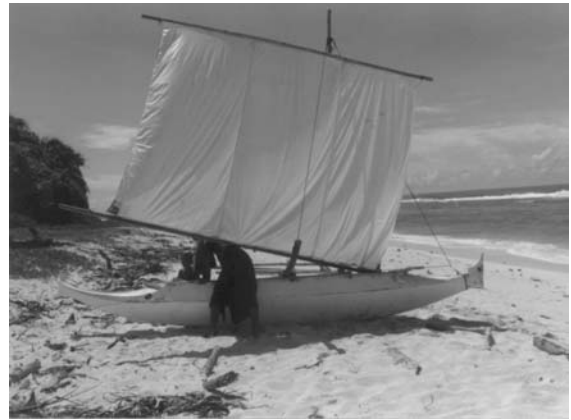
Seafaring in the Polynesian Outliers. Fig. 6 Outrigger canoe of vaka pai manu type, rigged with rectangular sail, on beach at Anuta island.
